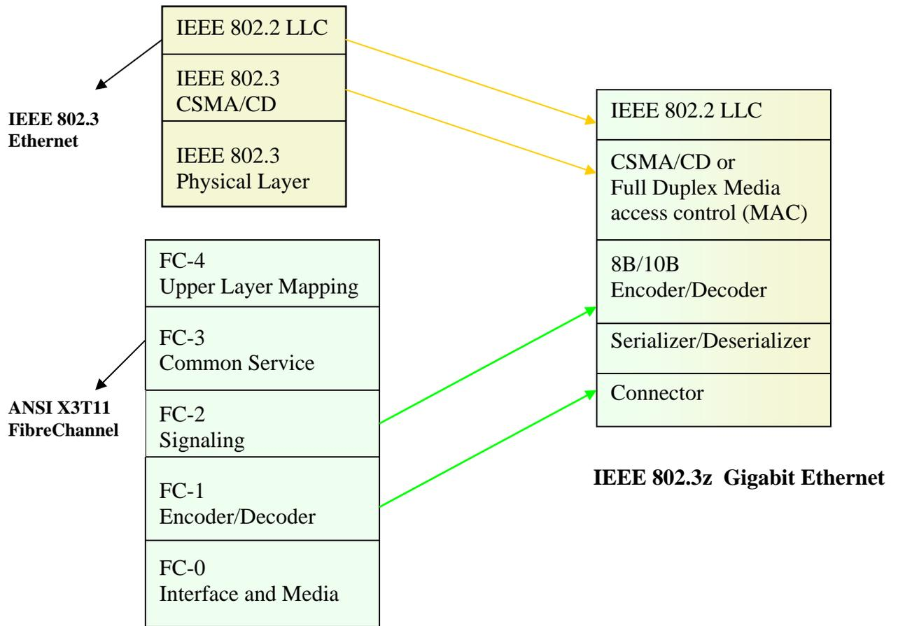
Figure 5.6.6 Gigabit Ethernet Architecture -1
