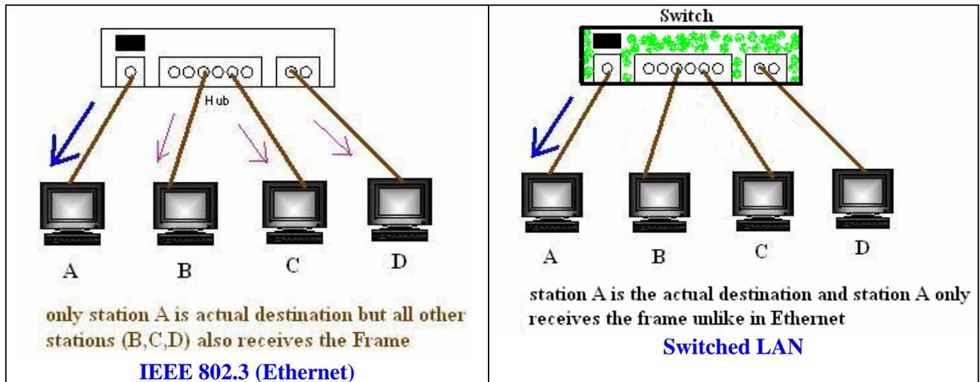
Figure 5.6.1 Difference Between 802.3 and Switched LAN
