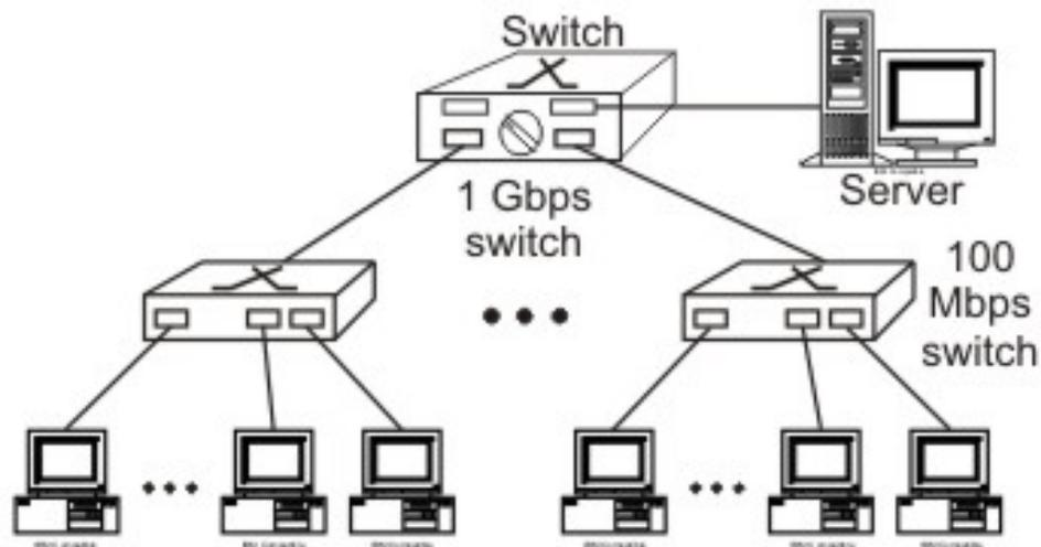
Figure 5.6.11 Migration to Gigabit Ethernet Backbone network
