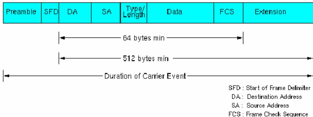
Figure 5.6.8 Ethernet Frame Format With Carrier Extension
