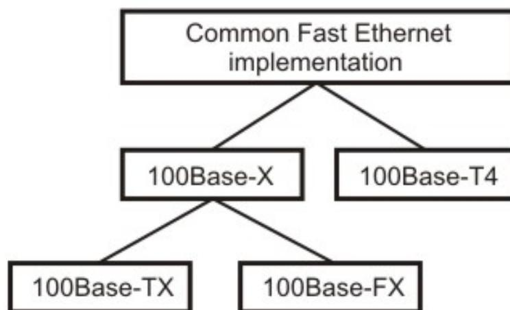
Figure 5.6.2 Fast Ethernet implementations
