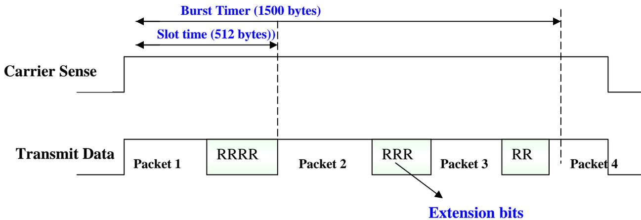
Figure 5.6.9 Packet Bursting
